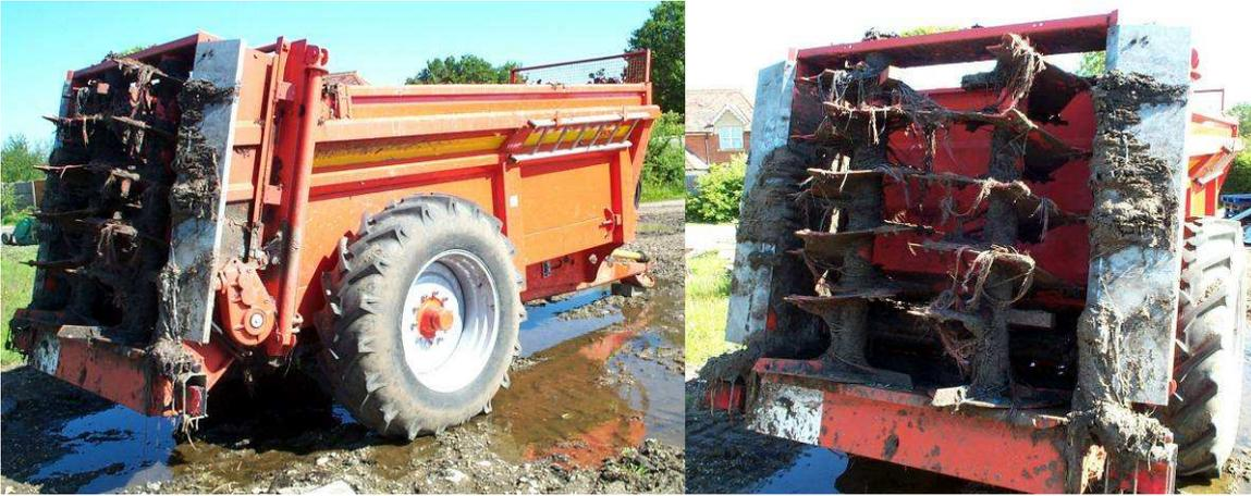
Figure 2. Rear discharge FYM spreader.
