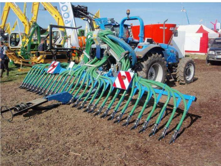
Figure 4. Umbilical system spreader
